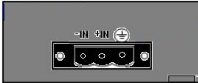
75W, -54.5VDC PoE Power Brick
